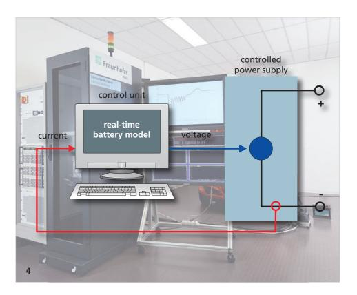
This leads to complex and time consuming battery pre-conditioning and testing processes. Virtual batteries reduce development times significantly.
